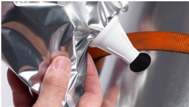
Foam moulding inside aluminium housing
