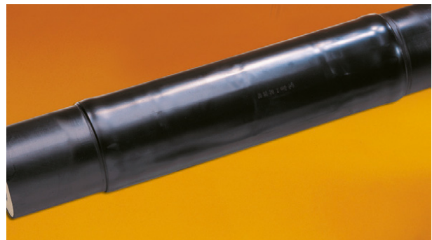
Correctly installed – the expansion marks have disappeared
